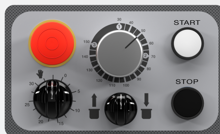
Variable speed control panel with electric up and down movement of the bowl
